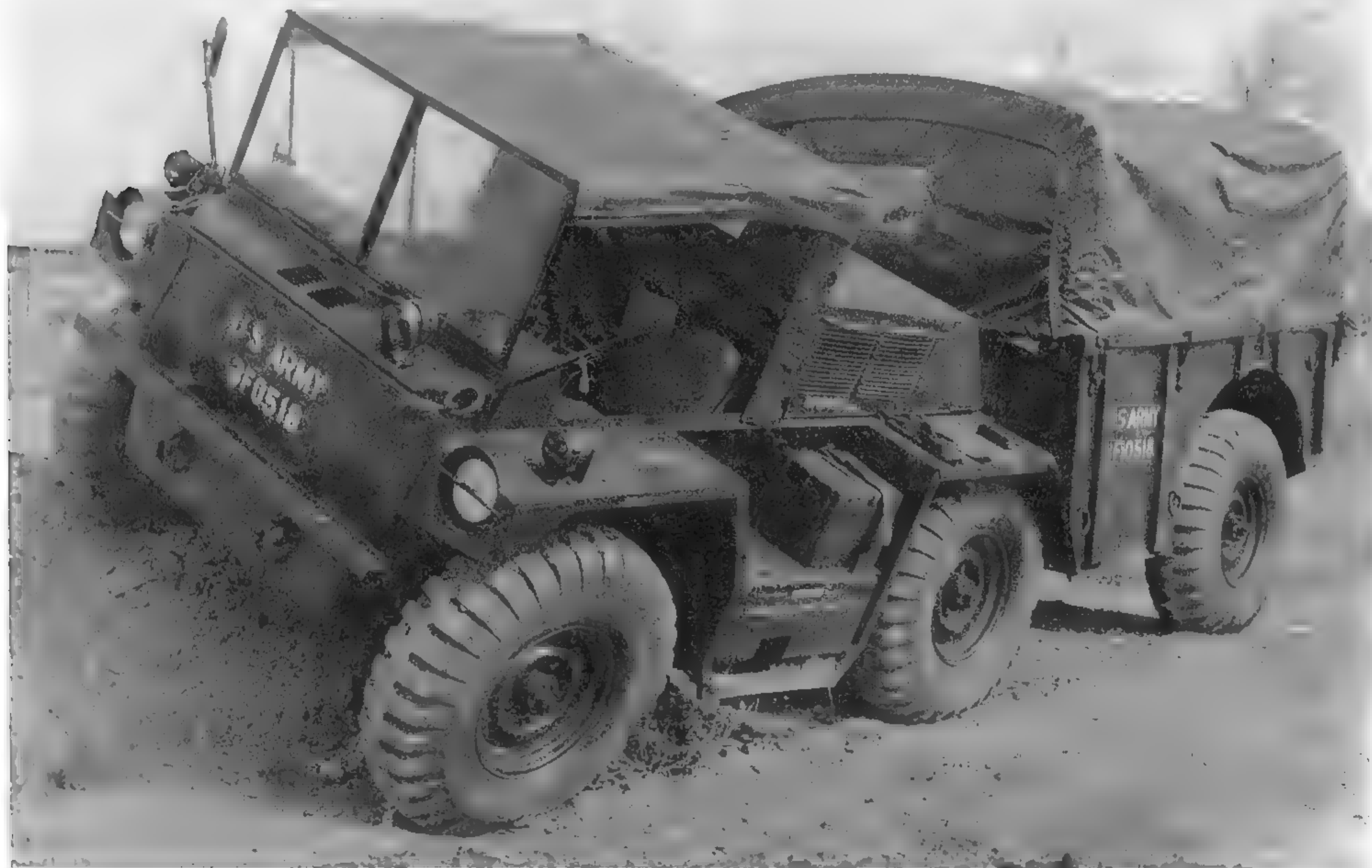
The Gama Goat has outstanding rolling flexibility. The early-type engine housing cover has an angular look. (U.S. Army photo)
